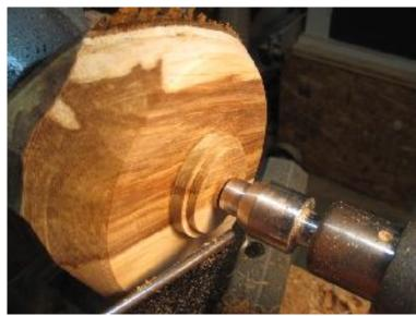
The step illustrated here serves a dual purpose. The smaller diameter tenon is what I'll actually grip the piece with in my scroll chuck. The larger diameter serves as a seat for the top of the chuck's jaws. This section will eventually get turned away and form the "neck" of the pedestal foot.
