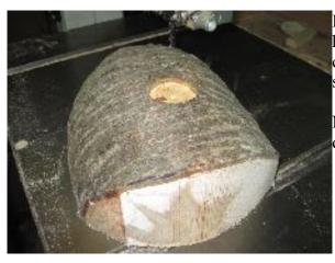
I've cut my blank on the bandsaw and drilled a 1 3/8" hole through the bark into the more solid sapwood in the center of the blank to give me a good, safe seat for my spur center.
