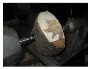
I begin turning at the tailstock end, removing the sharp edge of the blank and working diagonally from center out toward the outer edge of the bark.
