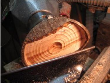
You can see that at about an inch deep I've still not cut down to solid wood. The sections that stick up (left and right in the photo) are the wings I've been discussing.
