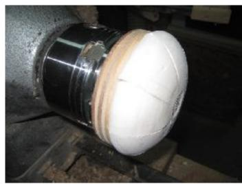
To finish the pedestal foot I'll be reversing the piece onto a jam chuck I made from some plywood and walnut. The jam chuck has a gently curved face covered with self-adhesive foam bought at a local craft store. I'll place the bowl over this and bring up the tailstock to "jam" it into place.
