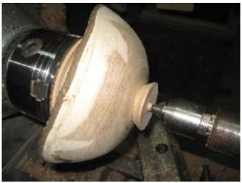
the foot, neck and the transition area of the bottom of the bowl at this time but the remainder of the sanding will take place off the lathe.
